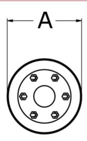
A = 90 D1 = 20 D2 = 40 L = 78 Nom. torque NM (Tkn) = 200
